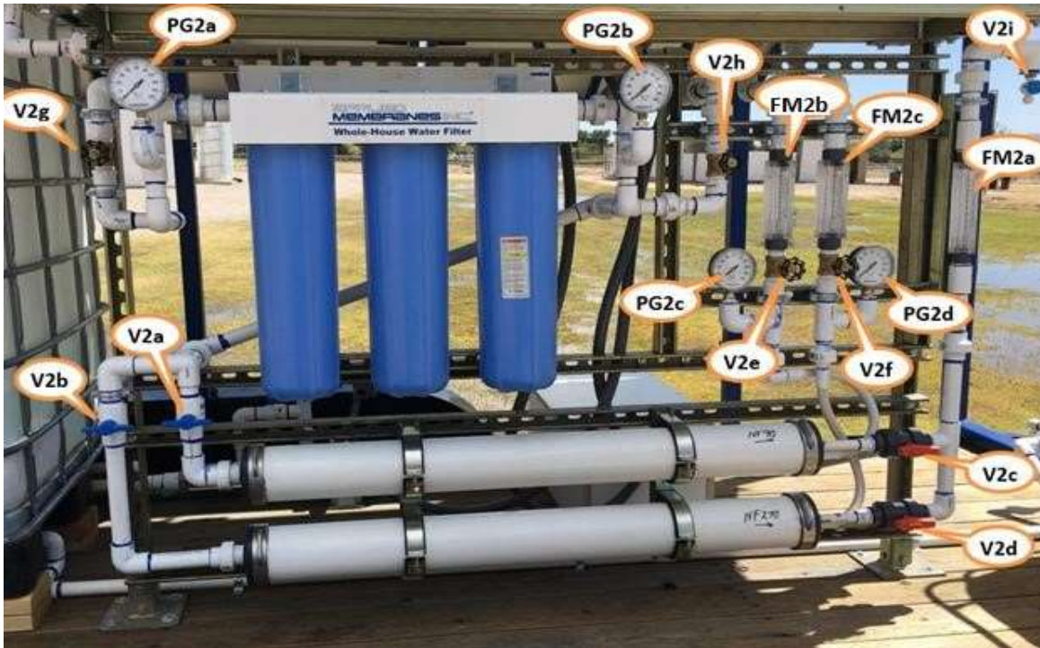
Figure 2. Side view of water purification system. The feed tank is at left and finished water tank is at right. The blue vertical cylinders are prefiltration units, and the horizontal cylinders house the NF membranes. Hinged solar panels are atop and behind (not shown). Valve (V), flowmeter (FM), filter (FT), membrane canister (M) and pressure gage (PG) positions are as indicated. Numbers correspond to figures where equipment is shown. The same designations are used in the text and tables.
