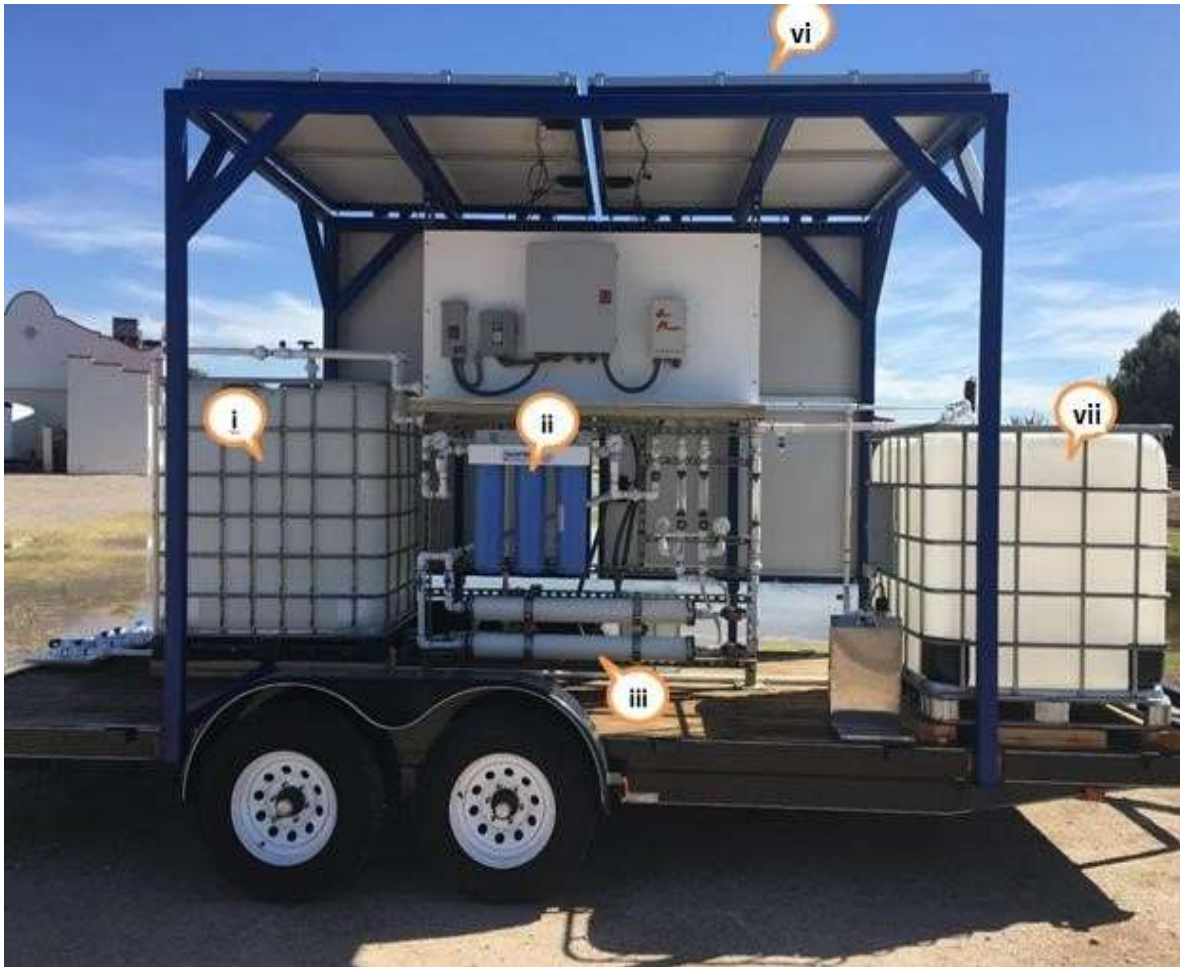
Figure 1. Full front view of the mobile, solar-nanofiltration system. The system consists of (i) a raw water tank (at left), (ii) prefilters (blue, vertical) and (iii) nanofiltration canisters (horizontal, white), (iv) electrical control system (top front, boxes), (v) direct current pump and battery array (not visible) (vi) solar panels (top and back) and (vii) finished water tank (at right).
