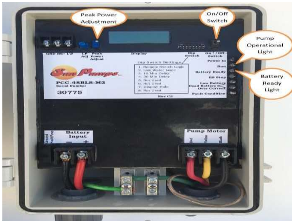
Figure 6e. Pump control unit. Pump readiness is indicated by a green light on the battery ready indicator. The toggle switch turns the pump on and off. Pump speed is controlled by the peak power adjustment screw (shown).
